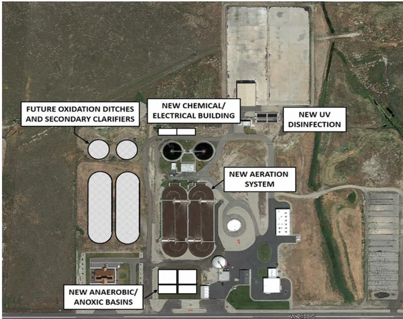
**PLAN VIEW OF BIOLOGICAL NUTRIENT REMOVAL AND UV DISINFECTION**
