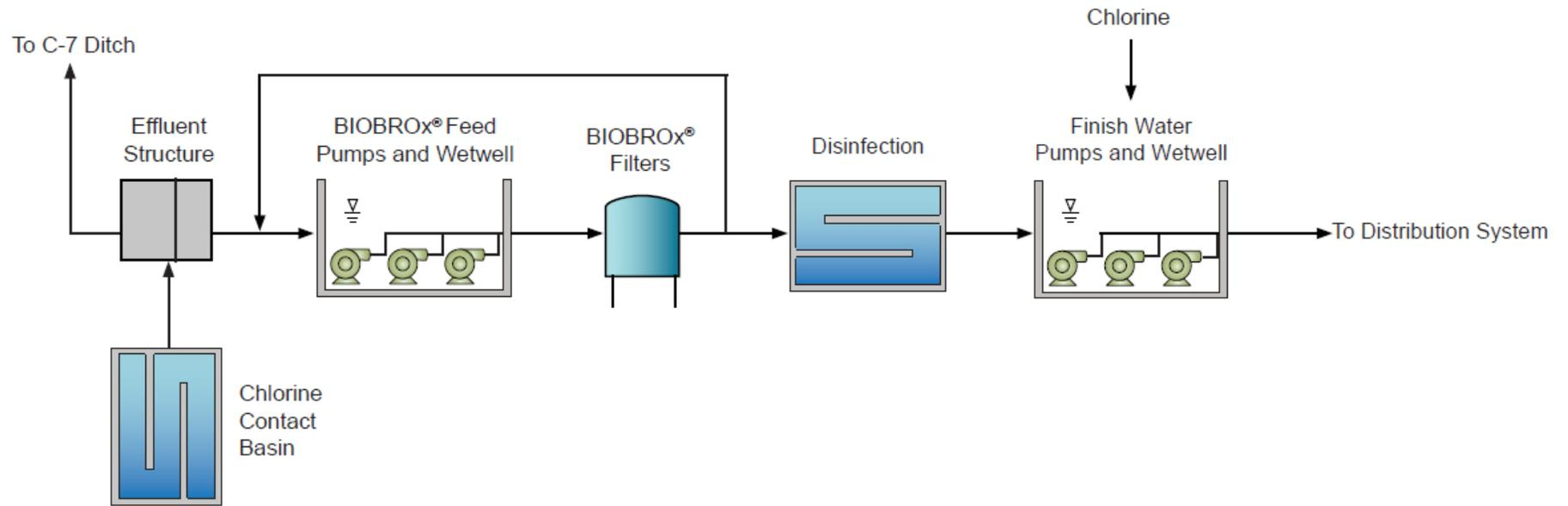
Figure 6 Secondary Reuse: BIOBROx®
