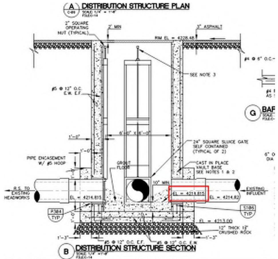
Figure 3 Distribution Structure Invert Elevation
