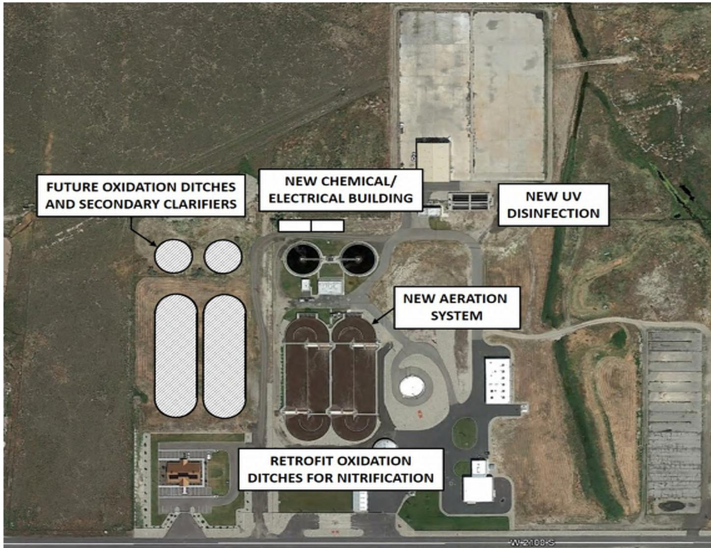
**PLAN VIEW OF NITRIFICATION WITH UV DISINFECTION**
