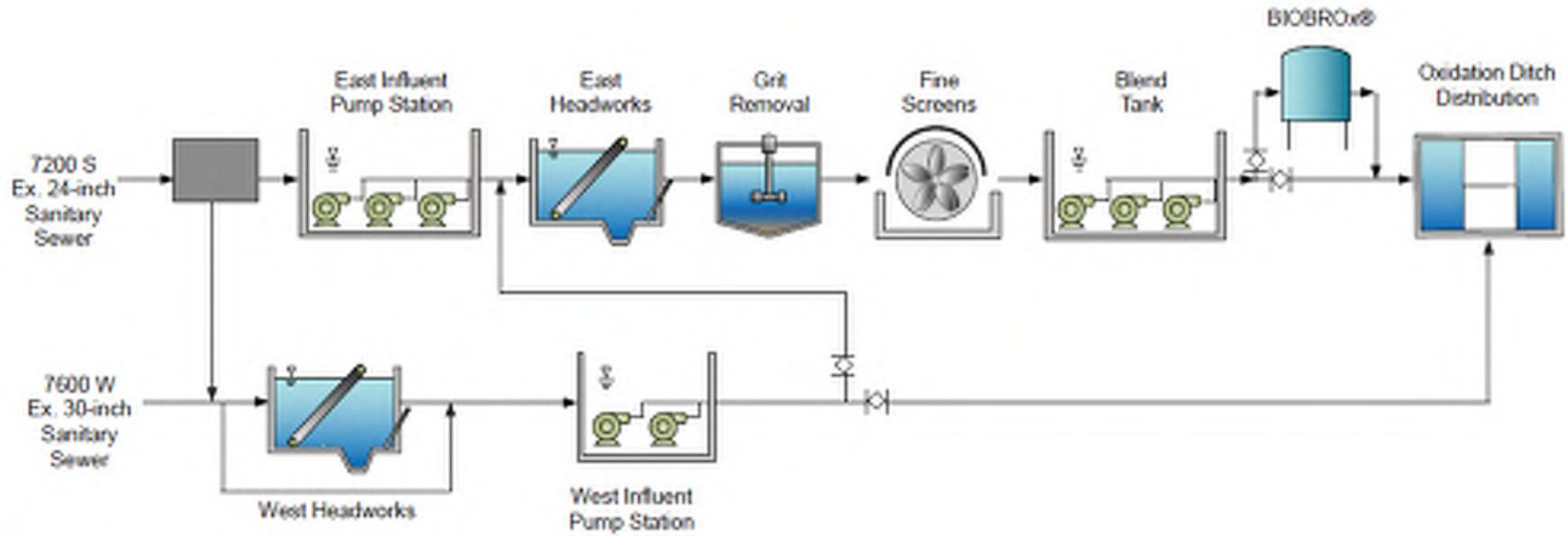
Figure 1 Existing Primary Treatment Schematic
