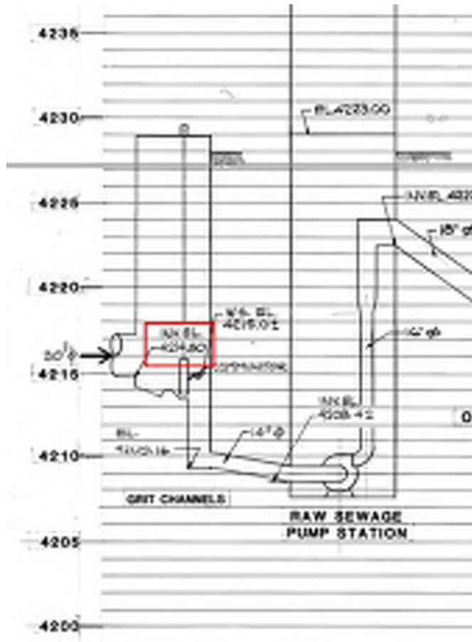
Figure 2 30-inch SS Invert Elevation
