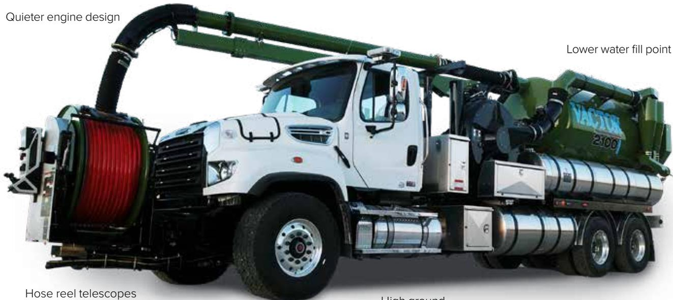
Hose reel telescopes out up to 15" and rotates up to 270° for optimal positioning
