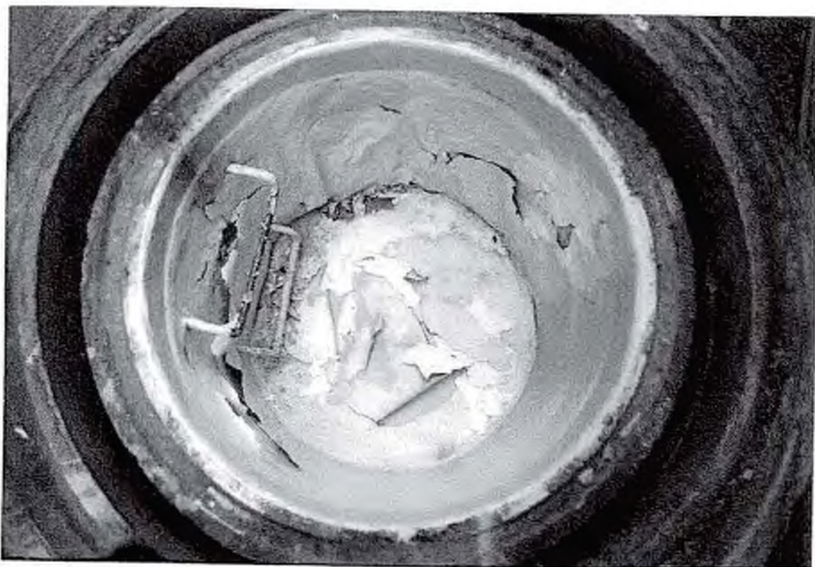
Figure 7. Epoxy coating failure.
